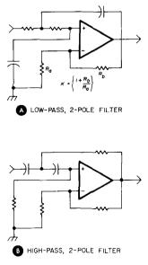
fig. 2. Basic op amp circuits for 3 dB low- and high-pass filters. Center frequency,  $f_0 = 1/2\pi RC$ , where network R and C are equal.
